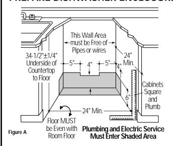
The rough cabinet opening must be at least 24" deep, 24" wide and approximately 34-1/2" high from floor to underside of the countertop. • The dishwasher must be installed so that drain hose is no more than 10 feet in length for proper drainage.
